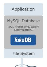
TokuDB is designed to be a drop-in replacement storage engine for MySQL and MariaDB. A software-only plug-in, TokuDB is ACID- and MVCC-compliant and is fully compatible with existing MySQL and MariaDB applications. It requires no modifications to existing code or application logic.
