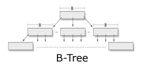
McCreight while working at Boeing Research Labs. The B-tree was developed to store huge amounts of data for fast retrieval on disk drives. The performance of the B-tree worked fine with the slow disks from 1970's era hardware.
